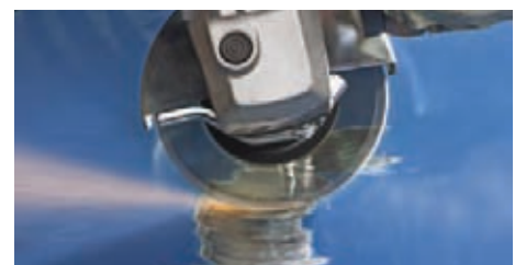
Grinding with Zebra slotted see-through disc: Good view of the material being processed
