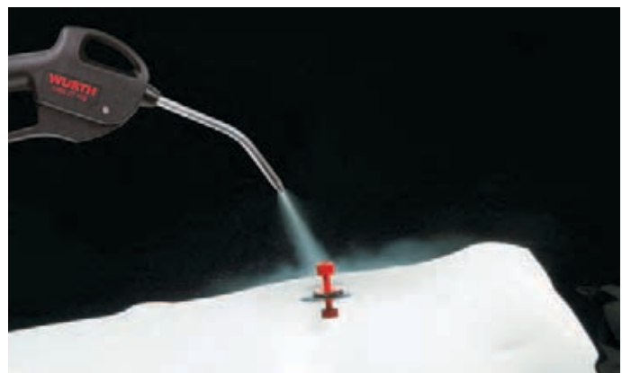
4. Cool the adapter off with compressed air or use WURTH Freeze Spray
