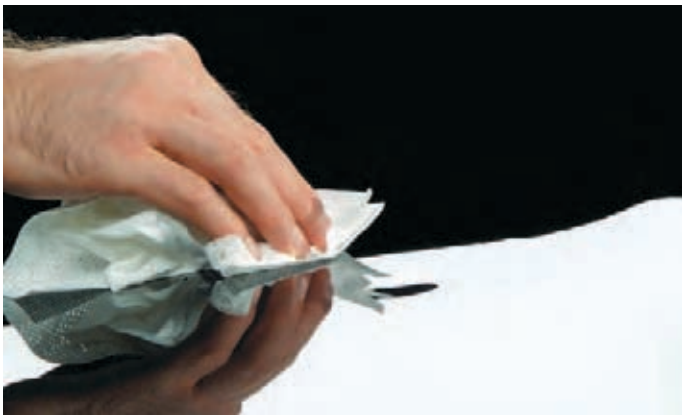
1. Clean dent with WURTH Clean Prep and, if required, affix a cross-mark
