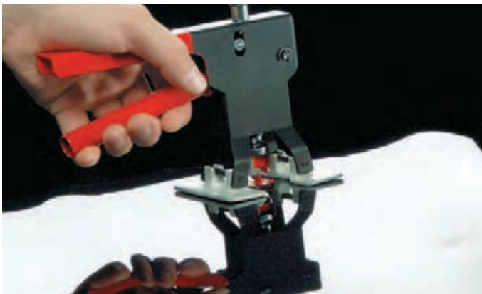
5. Attach the Mini Dent lifter to the adapter and carefully pull out the dent
